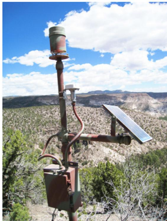
*OneRain's StormLink™ Satellite Telemetry installed in the Cochiti fire burn area in northern New Mexico. Real-time data is transmitted to OneRain's secure data storage center for web-based viewing, and 24x7 monitoring via Contrail®*
