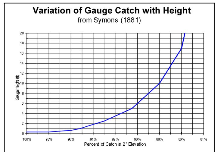
Figure 2: Variation of gauge catch with height for a given set of wind conditions as report by Symons (1881)
