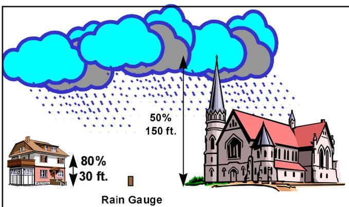
Figure 1: A demonstration in 1769 showed that a rain gauge located at the top of an 150 ft. abbey tower collected just 50% of the ground level rainfall and a gauge on the roof top of a 30 ft. house collected 80% of ground level rainfall.
