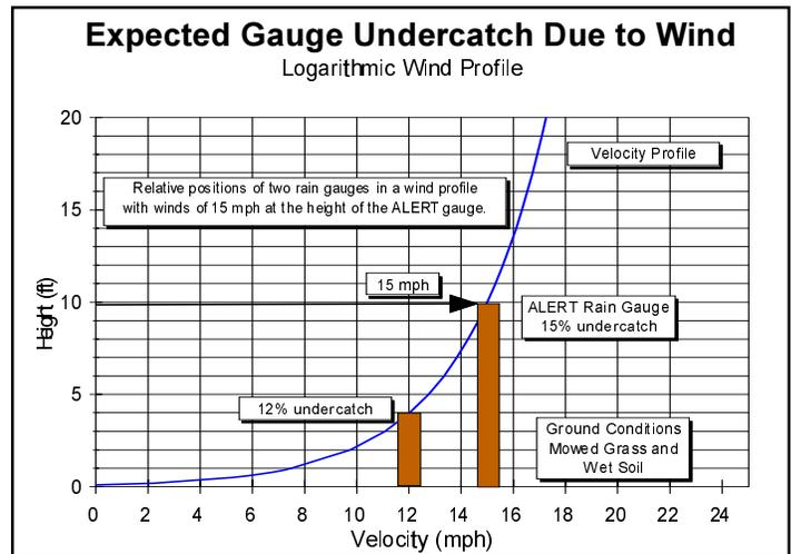
Figure 3: Expected gauge undercatch due to 15 M.P.H. wind
