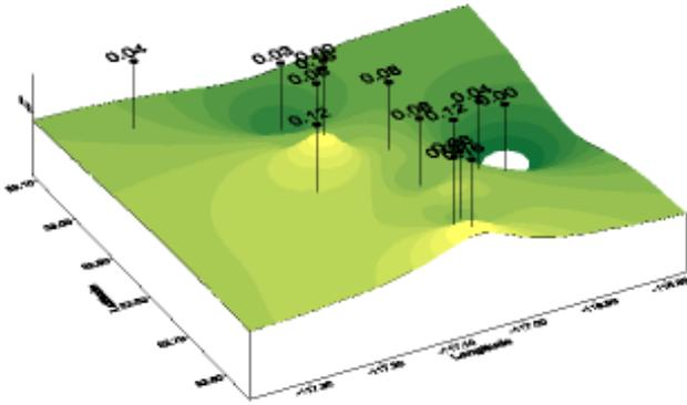
Figure 4: Rainfall contours derived from inverse distance squared weighting (Values are rain gage measurements in inches.)
