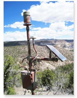
OneRain's StormLink<sup>™</sup> Satellite Telemetry installed in the Cochiti fire burn area in northern New Mexico. Real-time data is transmitted to OneRain's secure data storage center for web-based viewing, and 24x7 monitoring via Contrail®
